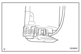
(b) Engage the 5 claw fittings and install the fuel pump onto the fuel pump case.
