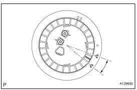
(2) Using SST, turn the retainer 740° to 760° clockwise (more than 2 turns), and position the mark on the retainer within range A to install it. SST 09808-14020 (09808-01410, 09808-01420, 09808-01430)
