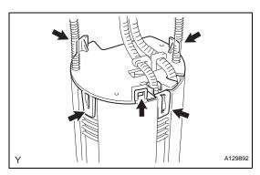
(b) Engage the 5 claws and install the fuel pump tank.
