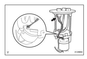
(c) Engage the clamp, then connect the connector.
